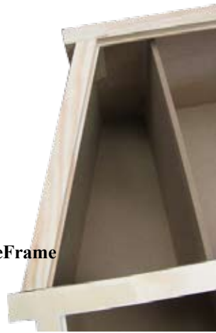
The Attic SideFrame's dado fits over the lip of the Rooftop Frame
